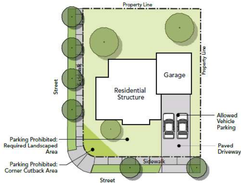
Figure 3-14 Single-Family Parking Location Requirements
